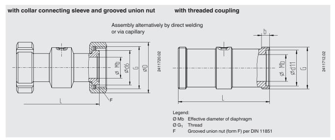
Pipe standard: Pipes per DIN 11866 row A or DIN 11850 row 2
